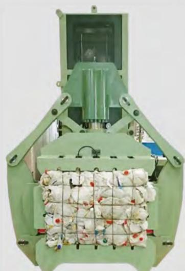
► The SCK Engineering Services range incorporates a specially designed rotating wire cutter that twists each wire before cutting. The twist design prevents the wires from slipping back, making the unit far more reliable, especially on expandable material.
