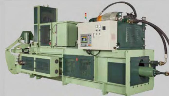
► The professional control panel incorporates a diagnostic, monitoring interface, easy to set operation parameters and varying material product changes. This function with fault finding locating device ensures ease of operation, troubleshooting and simple maintenance.
